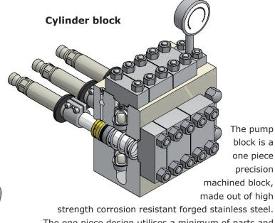
strength corrosion resistant forged stainless steel. The one piece design utilises a minimum of parts and seals, is fully sanitary and suitable for C.I.P.
